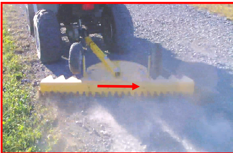
When set at 22 degrees, the ATR moves grading material from the sides to the center of the driveway.
