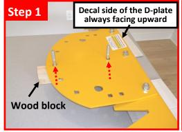
Place a support block under the curved edge of the D-plate. Insert the two <u>extra long</u> bolts up through the square holes in the D-plate.
