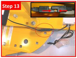
Connect the power wire from the 12 volt actuator to short wire from control box.
