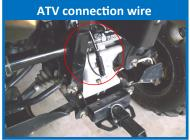
Red Banded wire (with white stripe) <u>must</u> be connected to the Positive (+) terminal of the battery.
