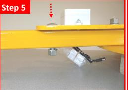
Inset a long bolt down through the rectangular hole in the front of the upper plate as pictured. Add washer and nut.
