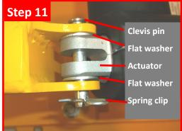
The front "power cord" end of the 12 volt actuator is connected to the actuator mount as pictured.
