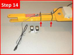
Secure the long wire from control box to the tongue tube with long zip ties.
