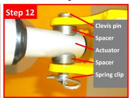
The back end of the 12 volt actuator is connected to the actuator mount as pictured.
