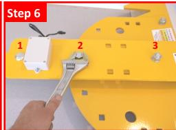
Finish tightening the three bolts with a 15/16 inch, or 24mm wrench, or large adjustable wrench.
