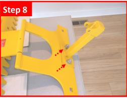
Secure the rear actuator mount by inserting two short bolts up through the square holes of the swing arm as pictured. Add washers & tighten nuts with wrench.
