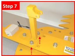
Secure the front actuator mount by inserting two short bolts up though the front set of square holes of the top plate as pictured.
