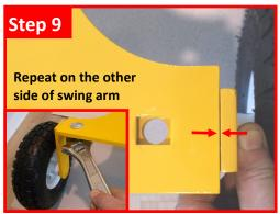
Positioning the top of the wheel assembly against one side of the swing arm. Insert its short bolt down through the rectangular hole. Add washers & tighten the nuts.
